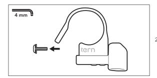
2. Remove the Body Adjustment Bolt.
