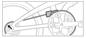
5. Place the Chain back onto the Chainring and then shift the Chain to the largest cog in the rear.
