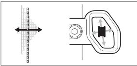
Shift through all gears to ensure that the Chain does not touch the Chain Guide Cage.
