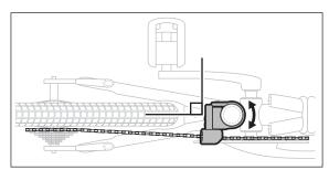
Align the Chain Guide Body so that the bottom of the Clamp is perpendicular to the bike.
