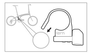
Mount the Chain Guide Body onto the Seat Tube and loosely tighten the Body Adjustment Bolt.
