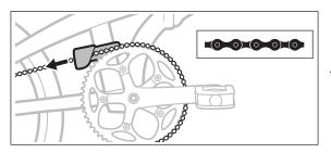
4. Route the Chain through the Chain Guide Cage and reattach the Chain.
