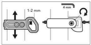
Adjust the Chain Guide Body so that the top
