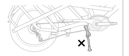
**3.** Position Master Link on the chain between Chain Guide Pulley and Motor.
